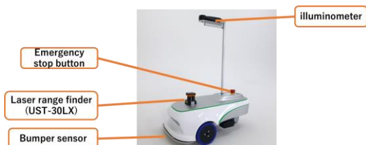
Fig. 1 Mobile robot for illuminance measurement
